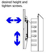
Adjust mount support horizontally and vertically by using the slots
