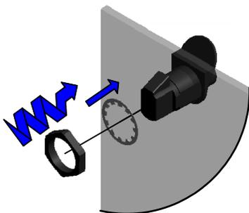
Slide and twist the Lock Washer and Nut (R), respectively, onto Cylinder (U) as shown in diagram. Ensure that it's placed in the correct position as shown in the diagram.
