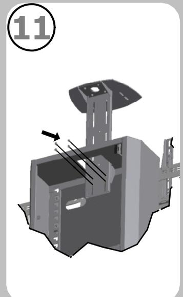
Attach acrylic (F) to camera bracket (D). Secure bracket (D) to body (A) at desired height using bolts.
