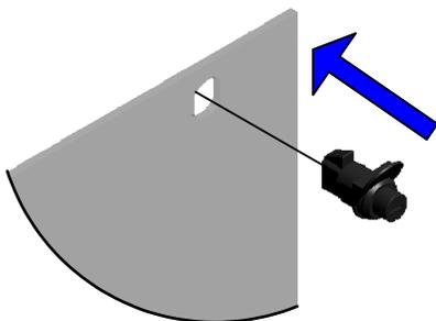
Slide Cylinder (U) through hole in glass as shown in diagram.
