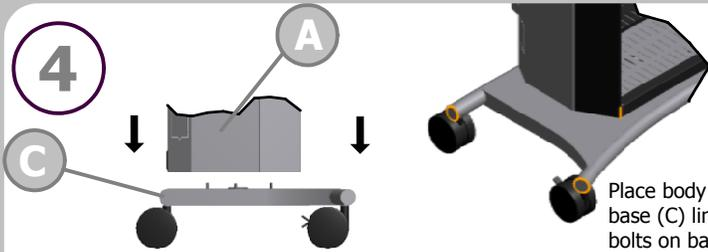
Place body (A) on base (C) lining up bolts on base with holes on body.
