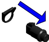
Slide Pull (T) over Cylinder (U). The Flange must be as shown in the diagram
