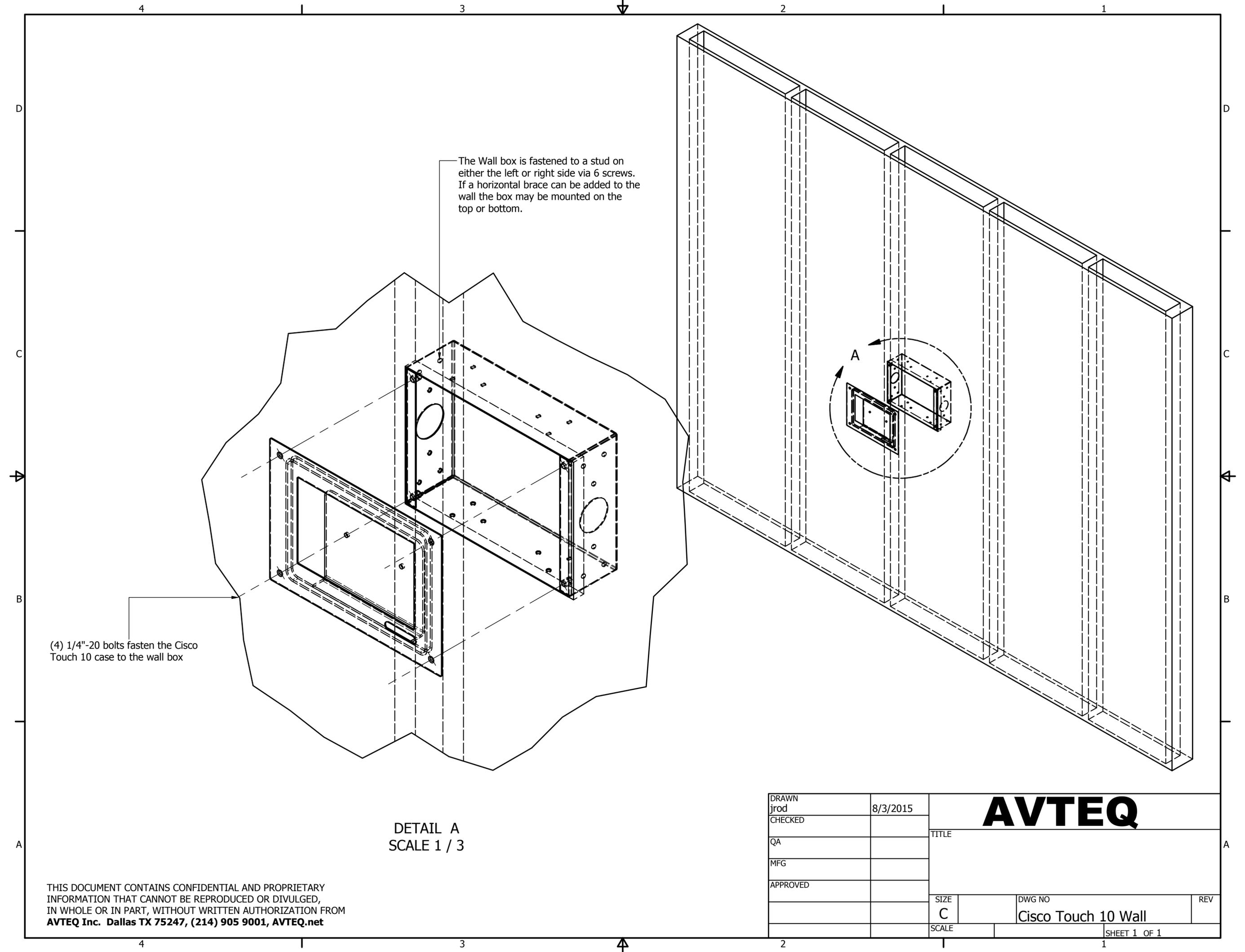
The Wall box is fastened to a stud on either the left or right side via 6 screws. If a horizontal brace can be added to the wall the box may be mounted on the top or bottom.
