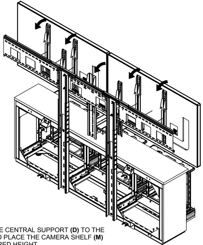
ATTACH THE CENTRAL SUPPORT (D) TO THE MOUNT AND PLACE THE CAMERA SHELF (M) TO DESIRED HEIGHT
