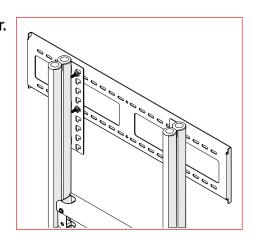
Mounting the 40/26" Omega (A) to the cart provisions with the 5/16" Screw, place a 5/16" washer on the front and a 5/16"washer on the back and tighted with the flange nut on the back. (5/16" harware included on the cart harware)
